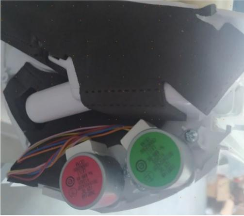
The STEPPER MOTOR moves the louver up and down, or right and left, depending upon selections made at the remote control.
