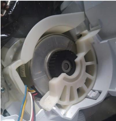
The Fan Motor is a variable speed motor. The air volume will vary with the speed of the compressor, or it can be set at the remote control to maintain a single speed.
