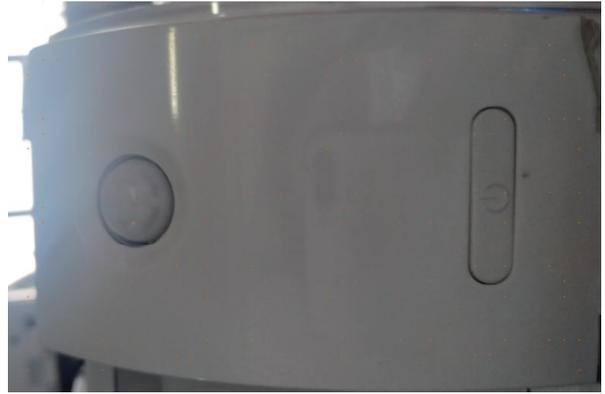
If the remote control is non-functional, the Emergency Button can be used. 73 -78 degrees will be maintained, until commands are received via the remote control.
