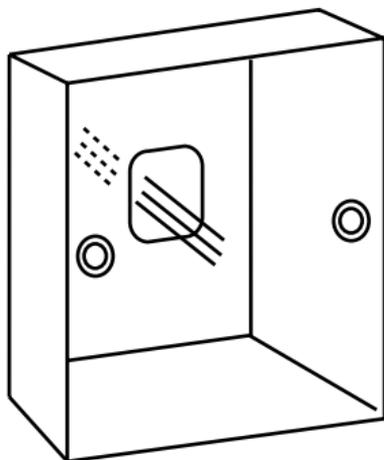
2. Fix back cover to the holder. After that, connect communication wire to CON1 port of wired controller. Finally put the front cover of wired controller to back cover to complete the installation.
