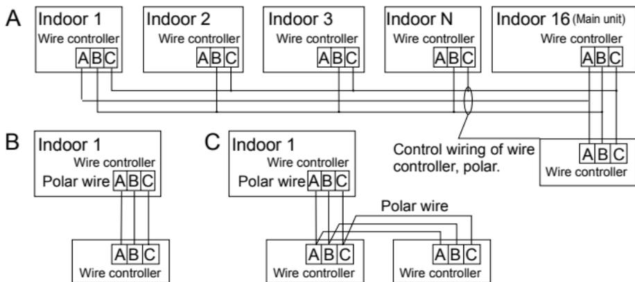
There are three methods to connect wired controller with the indoor units
