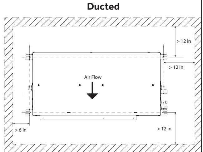
(1) Single-unit installation (unit: in. (mm.))
