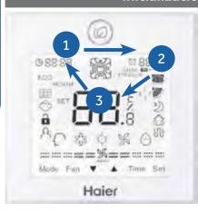
The wired controller will momentarily display all display icons upon powering up or when resetting the system.
