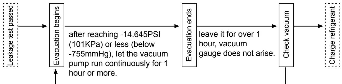
if vacuum needle rises, it shows there is water or leakage in the system, please correct the problem and then evacuate again.
