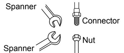
If threading the nut as not aiming at the center, the screw thread will be damaged, further it will cause leakage.
