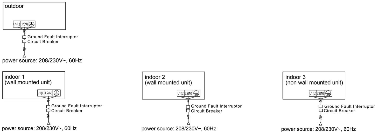
Indoor and outdoor use their individual power source. All indoors use one power source. Must install the leakage breaker and the over current breaker, or electric shock will occur.
