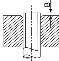
Projecting length of pipe to be expanded: B(mm)
