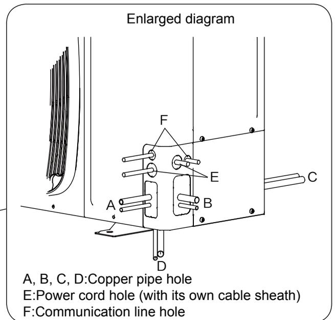
As shown in the figure, the piping can be connected from four directions. Through the front / rear hole piping piping on the cover hole or crack directly across the floor.
