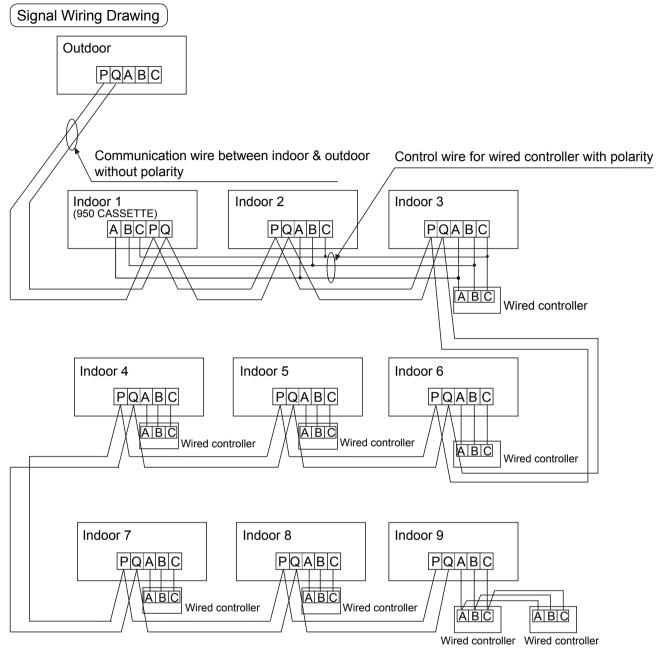
Outdoor units are of parallel connection via three lines with polarity. The main unit, central control and all indoor units are of parallel connection via two lines without polarity.
