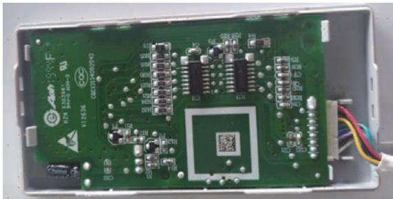
The indoor display has an infrared communication circuit that receives operating commands from the remote control. This display will indicate operating modes, error codes, indoor air temperature, timer status, and power status.
