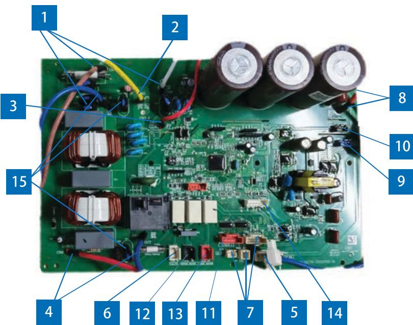
**PCB (2) (Module PCB for 09K )**
