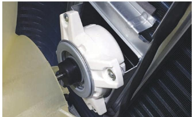
The fan motor is a variable speed motor. The required speed is calculated by the PCB. The motor is electrically connected to the PCB via PLUG CN-21.
