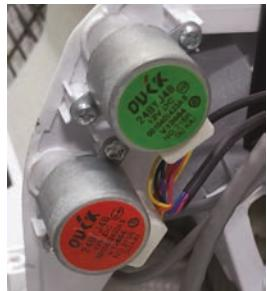
The STEPPER MOTOR 1 and 2 moves the louver up or down, depending upon selections made at the remote control.
