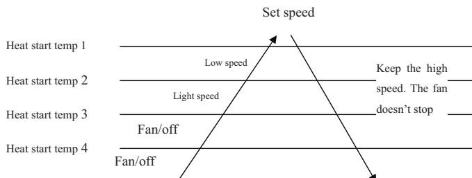
4 minutes after the indoor fan starts, the light or low speed will switch to the set speed.
