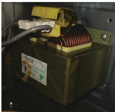
The Reactor is a power filter. It is unlikely to ever have an electrical failure of this component.
